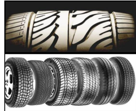
A tyre having a tread depth which is less than 1.6 mm over the centre  $\frac{3}{4}$  of its breadth is deemed to be 'illegal' and constitutes a motoring offence.
